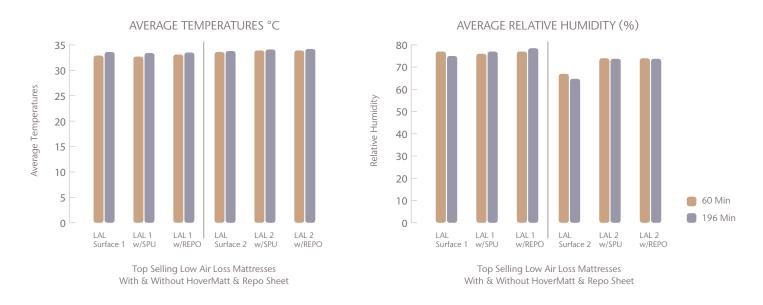
\*The data is calculated at a 95% confidence interval. Adapted from Heat and Water Vapor Testing (Body Analog Test Method), Project #1710 - EC Service, Inc. Data on file at HoverTech International.
