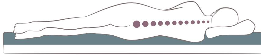
**Description:** Results of the immersion test method indicate how far a load sinks down into the support surface. It depicts the potential for pressure redistribution.
